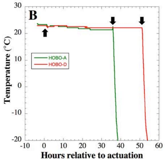
Figure 4. (A) Actuation of BRIC-23 canisters onboard the ISS by astronaut Jeffrey Williams. (B) Temperatures recorded during BRIC-23 flight for *B. subtilis* (HOB0-A, green line) and *S. aureus* (HOB0-D, red line). Time of actuation is denoted by upward arrow, and time of canister transfer to the onboard  $-80^{\circ}\text{C}$  freezer is denoted by the downward arrows.
