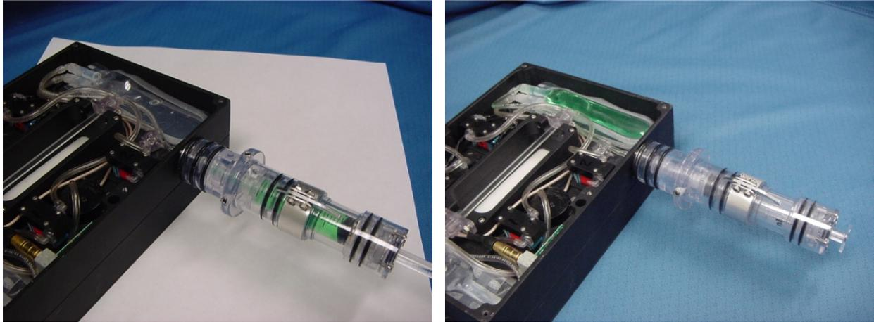
Figure 2. Left: a photograph of the Transfer Tool engaged to the Needle-less Septum Port prior to the sample input (see also image in Figure 3). Right: After being emptied into the cassette bag.
