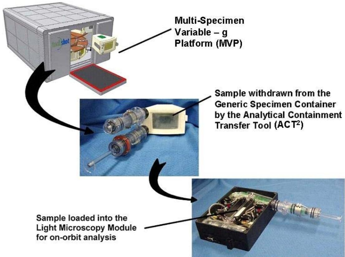
Figure 3. Example of an application of the Double Containment Transfer Tool: Transfer of biological suspensions between an experiment facility, such as a variable-g centrifuge with culture modules equipped with a needle-less septum port, and a receiving cassette for microscopy.
