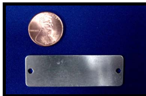
Figure 2. Aluminum coupon used in surface treatment testing.
